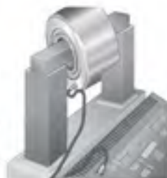
Heating with an induction heater
